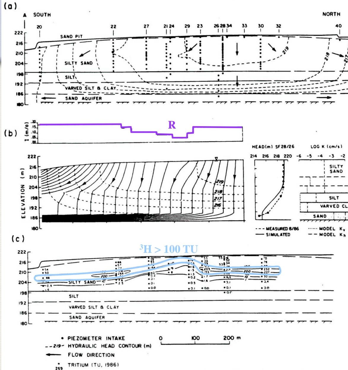
Fig. 3. Section A-A': (a) hydraulic head measured, August 1986. (b) simulated flow net, showing water table recharge rate and K layering used for simulation, and (c) tritium distribution.
